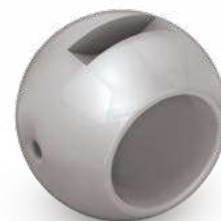
3 mm relief hole face the upstream
