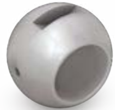
3 mm relief hole face the upstream
