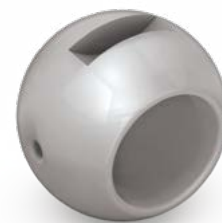
3 mm relief hole face the upstream
