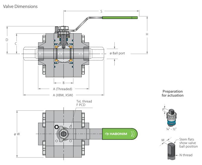
Face To Face of Flanged end connections are per flange standards, for other end connections consult us.
