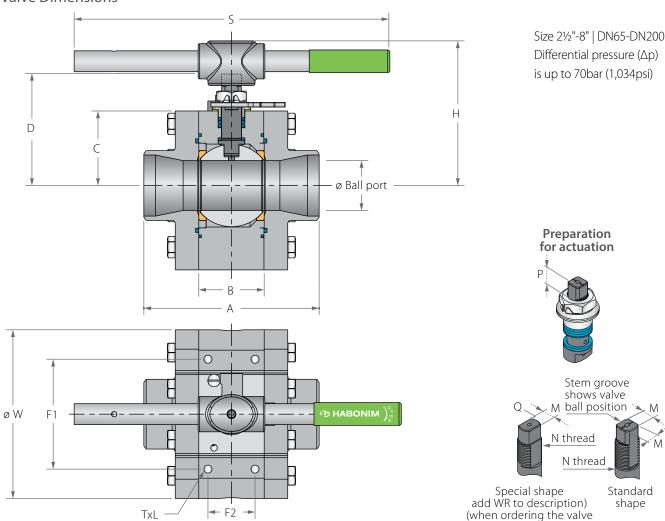
Face To Face of Flanged end connections are per flange standards, for other end connections consult us.
