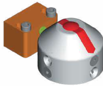
NAMUR VDI/VDE 3845 connection to limit switches
