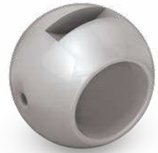
3 mm relief hole face the upstream
