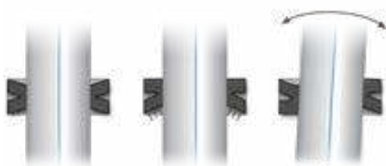
No pressure Pressure build-up Side load
