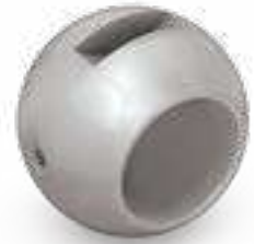
3 mm relief hole face the upstream
