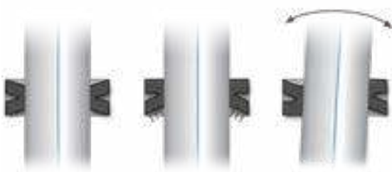
No pressure Pressure build-up Side load
