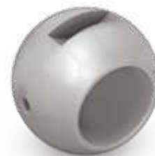
3 mm relief hole face the upstream
