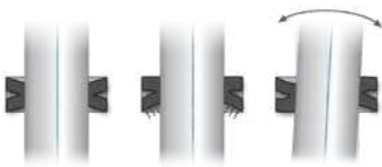
No pressure Pressure build-up Side load
