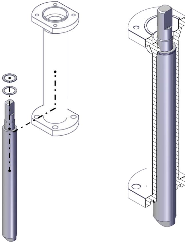
**Stem assembly for valve sizes 1/4"-2 1/2" (DN8-DN60)**
