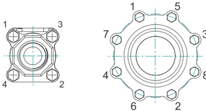
3.13. Tighten the body bolts according to **table 2**:
